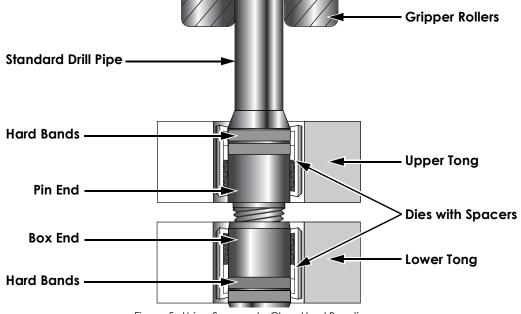
Figure 5: Using Spacers to Clear Hard Banding
