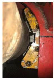
Figure 14: Right Hand Side Seated Dies
