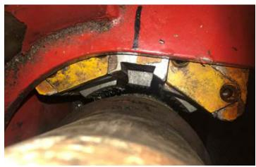
Figure 12: Clamps Slightly Closed
