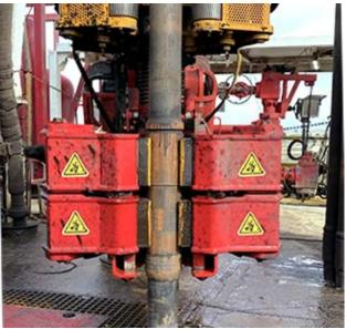
Figure 11: Tongs Aligned to Pipe Joint
