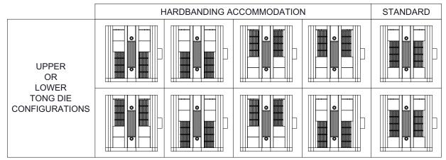
Figure 7: TM80/100 Die Configurations
