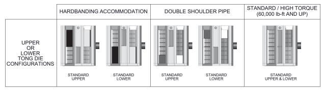
Figure 8: TM120 Die Configurations
