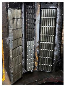
Figure 10: Dies Within Proper Wear
