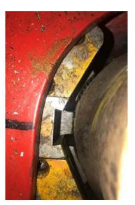
Figure 13: Left Hand Side Seated Dies
