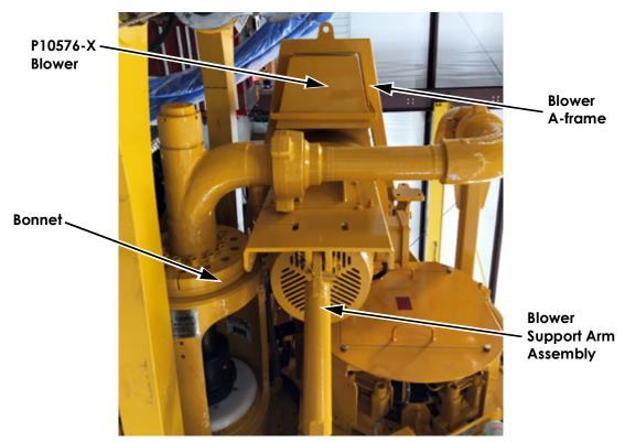
Figure 2: P10576-X Series Blower Configuration
