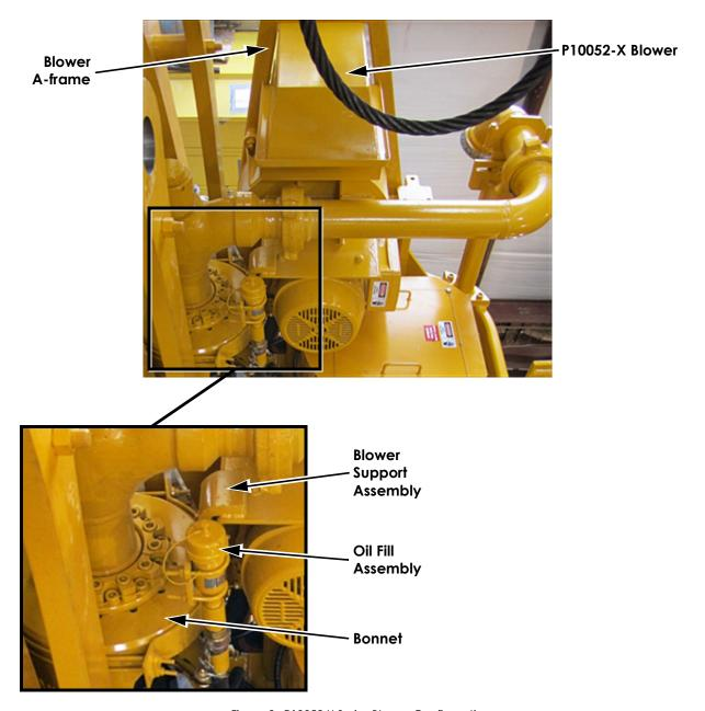
Figure 3: P10052-X Series Blower Configuration
