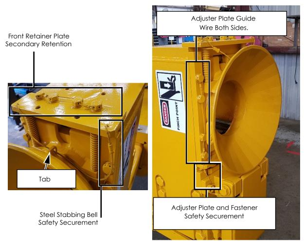
Figure 18: Front Retainer Plate and Stabbing Bell Lock Wiring
