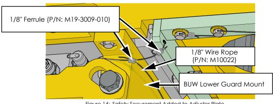
Figure 14: Safety Securement Added to Adjuster Plate
