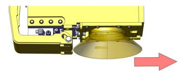
Figure 6: Slide the Steel Stabbing Bell toward the front of the gripper to remove
