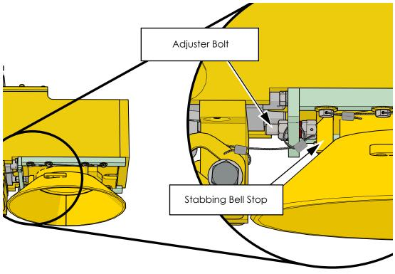
Figure 15: Stabbing Bell Adjuster Bolt
