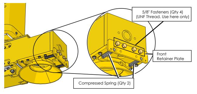
Figure 5: Loosen Fasteners uniformly to control the release of spring energy
