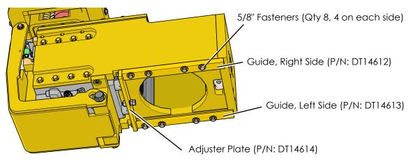
Figure 8: Back-Up Wrench with old design for Adjuster Plate and Guides
