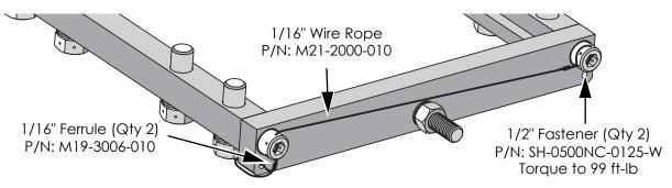
Figure 9: Safety Wire the bolts on the Adjuster Plate
