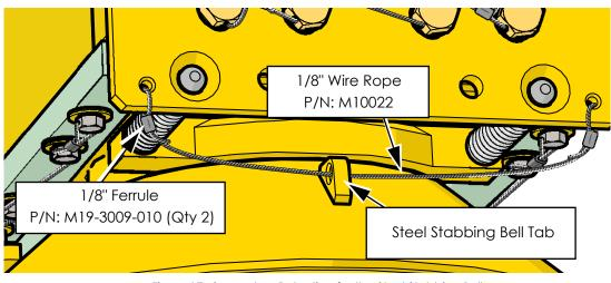
Figure 17: Secondary Retention for the Steel Stabbing Bell
