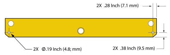
Figure 1: Modifying Existing Adjuster Plate (P/N: DT14614)
