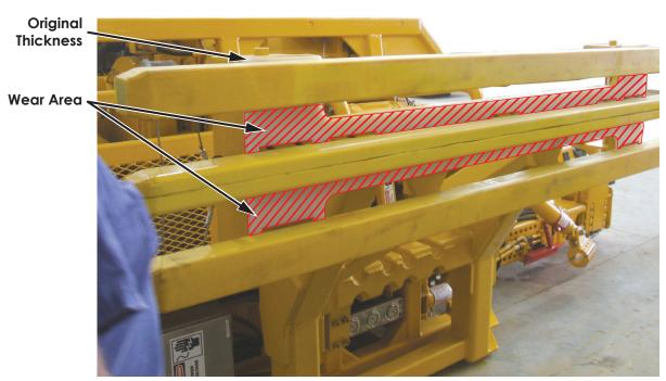
Figure 2: Measure Wear Pad in these Two Places
