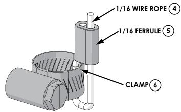
Figure 4: Crimp safety wire to Item 6 (hose clamp)
