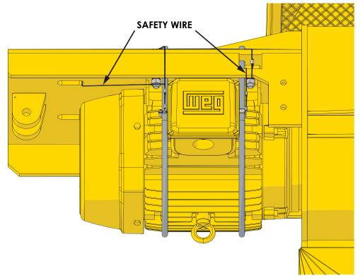
Figure 5: Safety Securement for U-Bolts
