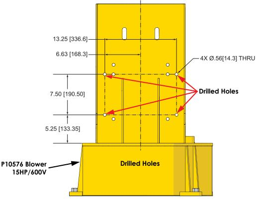
Figure 1: Four holes required to mount U-bolts on P10576 Blower
