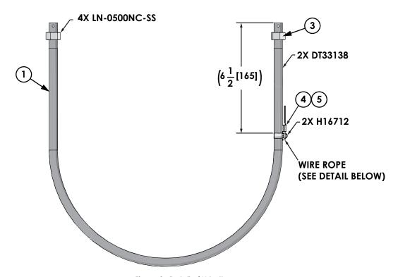
Figure 3: Detail of U-bolt
