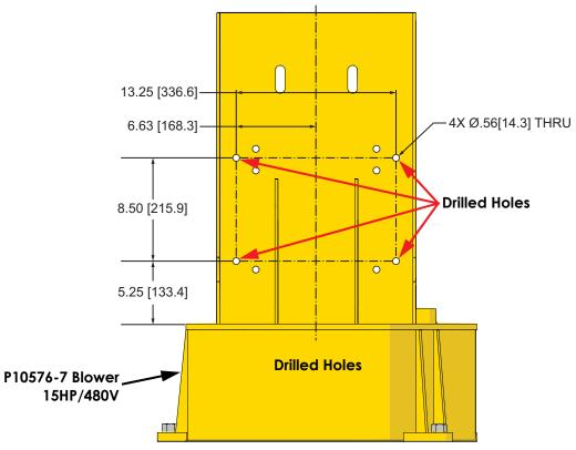
Figure 2: Four holes required to mount U-bolts on P10576-7 Blower
