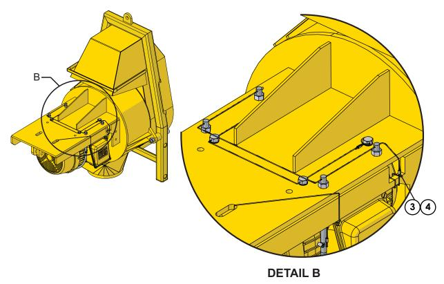
Figure 7: Safety securement on the U-bolts. See Table 1 on page 2 for items.
