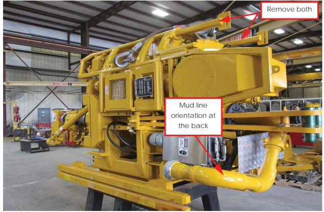
Figure 2: For top drives with the mud line orientation at the back of the top drive, remove both unused mud mounts and fasteners
