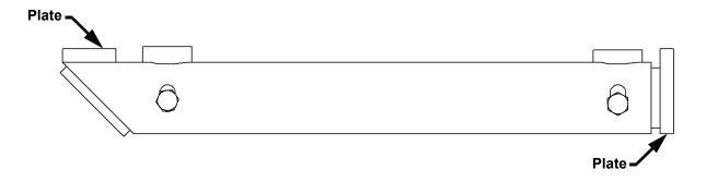
Figure 3: Limit Switch Guard with Plates
