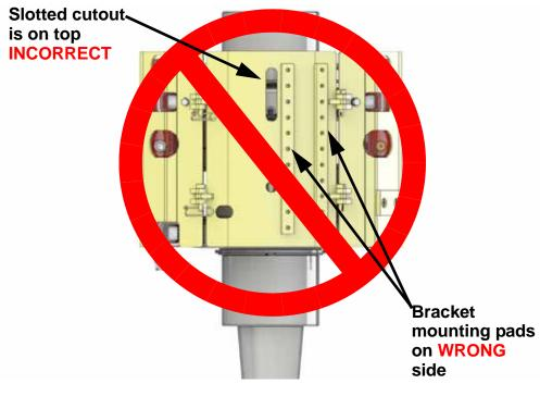
Figure 18: Straight-on view, **INCORRECT** guard panel orientation.
