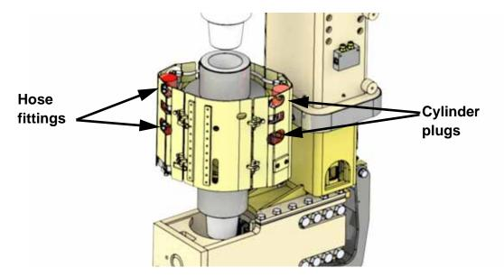
Figure 7: Angled view, correct LWCV rotation.
