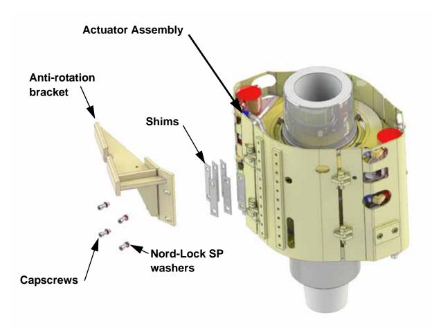
Figure 9: Anti-rotation installation.
