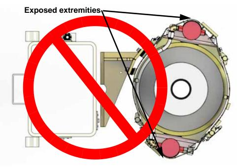
Figure 11: Top view, **INCORRECT** anti-rotation bracket installation.
