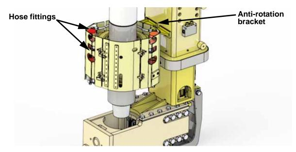
Figure 12: Angled view, correct installation of anti-rotation bracket.
