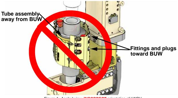
Figure 4: Angled view, **INCORRECT** orientation of LWCV.
