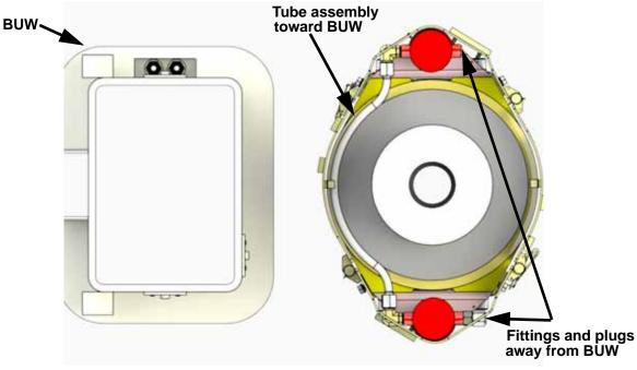
Figure 1: Top view, correct orientation.
