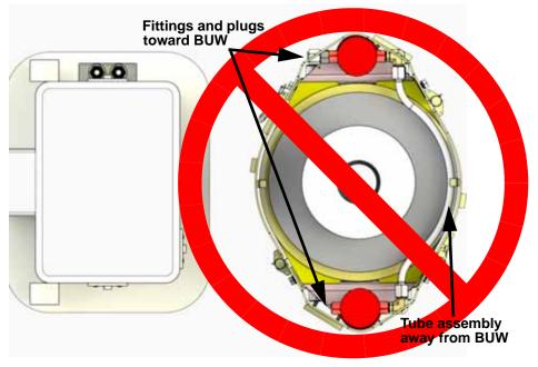
Figure 2: Top view, **INCORRECT** orientation of LWCV.
