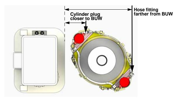
Figure 5: Top view, correct LWCV rotation.
