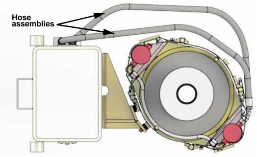
Figure 13: Top view, correct installation of hose assemblies.
