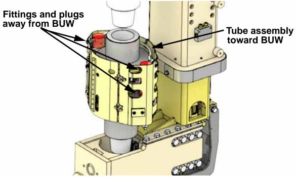
Figure 3: Angled view, correct orientation of LWCV.
