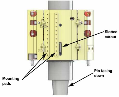
Figure 16: Straight-on view, correct guard panel orientation.
