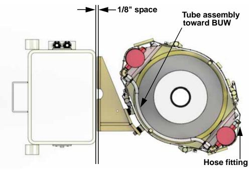
Figure 10: Top view, correct anti-rotation bracket installation.
