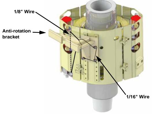
Figure 15: Secondary retention.
