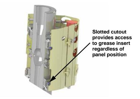
Figure 17: Section view, LWCV actuator assembly (correct guard panel orientation).
