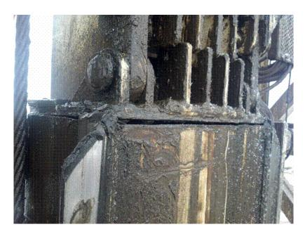
Figure 1: Cracked Portable Torque Guide Weld Joint
