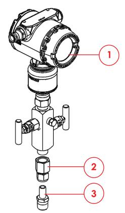
Figure 2: Transmitter assembly (with Swagelok fittings)
