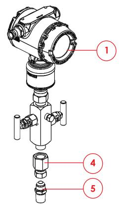
Figure 3: Transmitter assembly (with JIC fittings)
