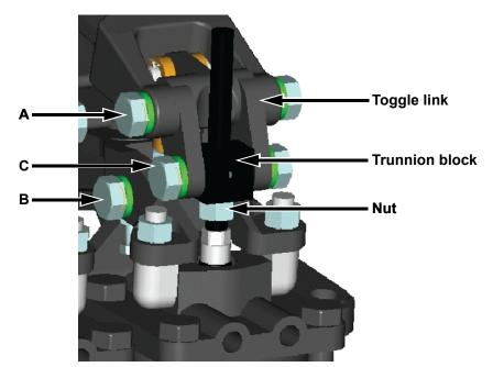
Figure 3: Toggle Link, Trunnion Block, and Nut
