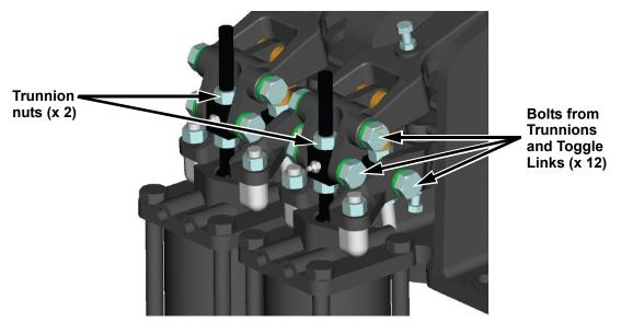
Figure 1: Trunnion and Toggle Links Nuts and Bolts
